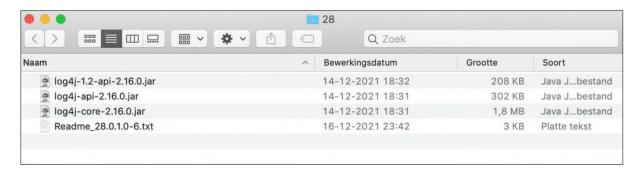
The top three files together form the patch for the vulnerability discovered in log4j.
